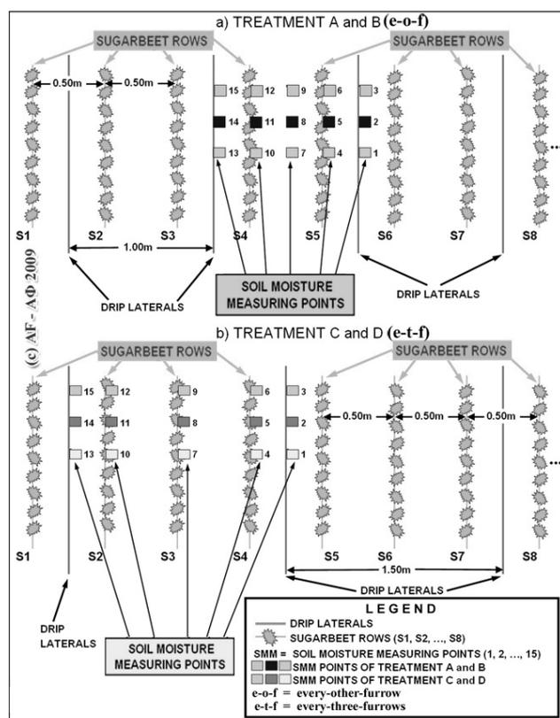
**FIGURE 3** a) Layout of the inline dripper lateral pipes of the plots of every-other-furrow (A and B). b) Layout of plots of every-three-furrows (C and D). Both layouts include the soil moisture measuring (SMM) points.
