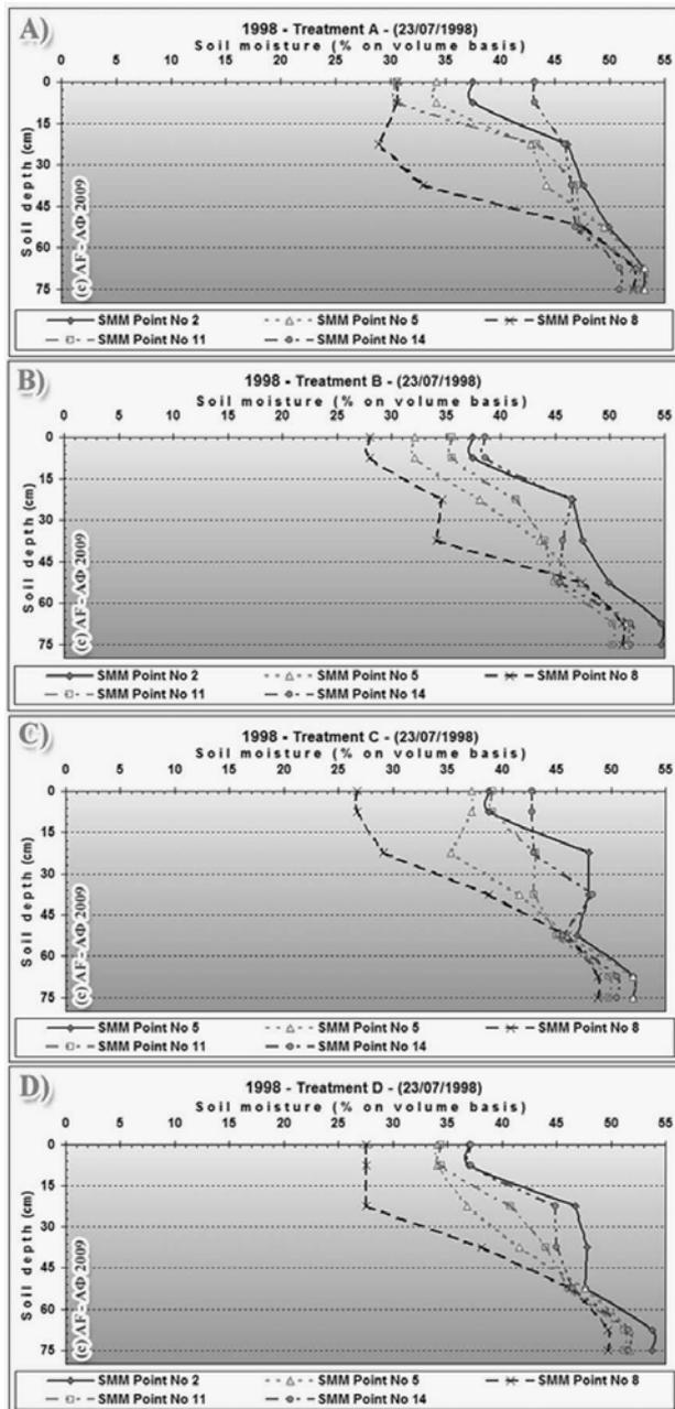
FIGURE 5 - Representative soil moisture distribution profiles for treatments A, B, C and D for the experimental plots of 1998.
