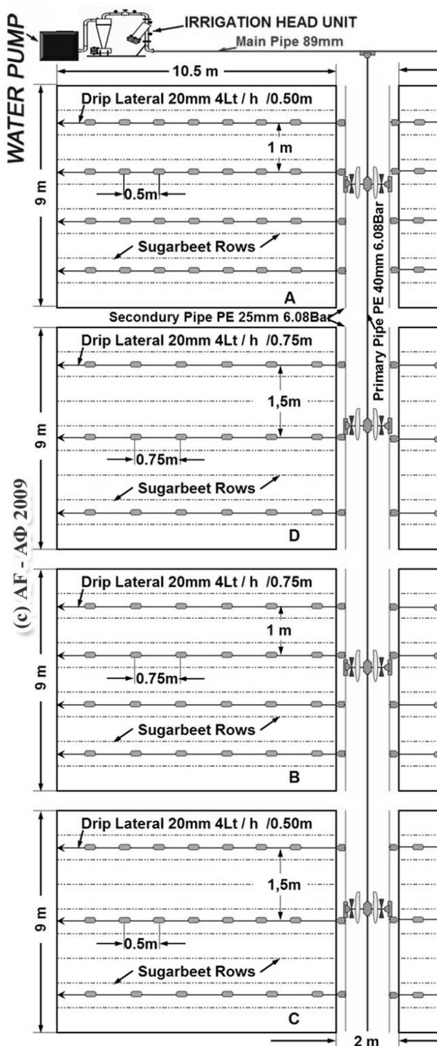
FIGURE 1 - Details of the layout design and of the drip irrigation system.
